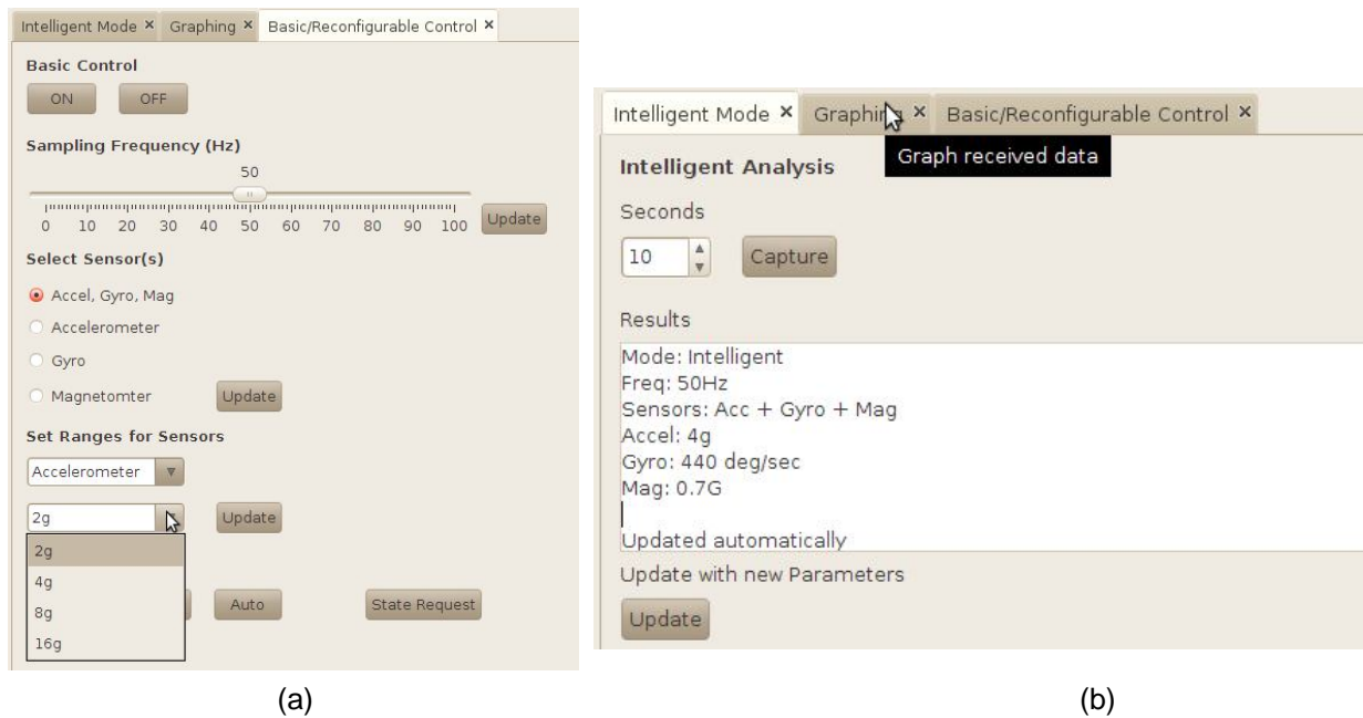
Figure 2. The Tyndall Wireless Inertial Measurement Unit (a) Reconfigurable mode, (b) Intelligent mode
