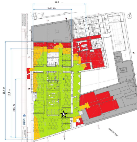
Figure 9. ZigBee 2.4GHz range test
