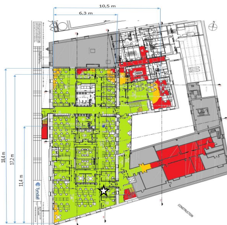
Figure 7. 868MHz range test
