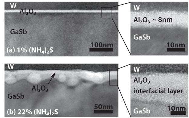
FIG. 2. Cross-sectional TEM micrographs of (a) 1% and (b) 22% (NH<sub>4</sub>)<sub>2</sub>S treated W/Al<sub>2</sub>O<sub>3</sub>/p-GaSb samples.
