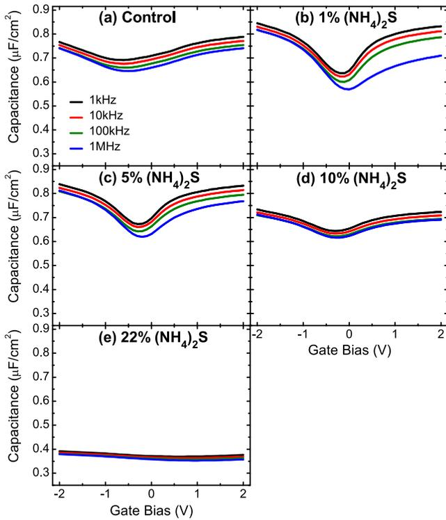
FIG. 1. Multi-frequency (1 kHz to 1 MHz) CV characteristics ( $\sim 295$  K) of Au/Ni/Al<sub>2</sub>O<sub>3</sub>/p-GaSb MOS capacitors with (a) no treatment (control) along with (b) 1%, (c) 5%, (d) 10%, and (e) 22% (NH<sub>4</sub>)<sub>2</sub>S treatments.
