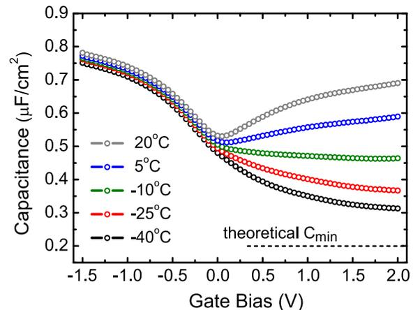
FIG. 3. 1 MHz  $CV$  response as a function of temperature ( $-40^\circ\text{C}$  to  $20^\circ\text{C}$ ) for Au/Ni/ $\text{Al}_2\text{O}_3/p$ -GaSb MOS capacitor treated with 1%  $(\text{NH}_4)_2\text{S}$ .
