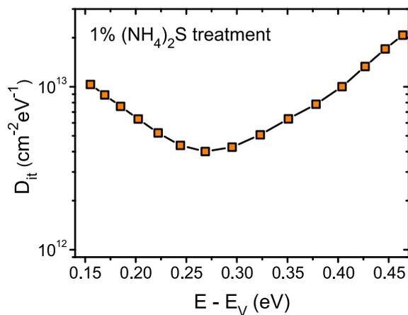
FIG. 4.  $D_{it}$  distribution from weak inversion towards the majority carrier band edge of 1%  $(\text{NH}_4)_2\text{S}$  treated sample extracted based on the temperature modified high-low frequency CV method.
