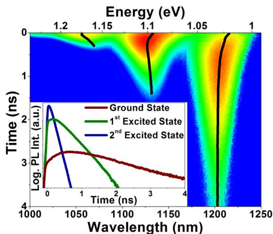
FIG. 3. Streak image [representing the logarithm of the emission intensity in color scale as a function of wavelength (energy) and time] measured at  $T = 10 \text{ K}$  under high-power density regime. The black lines show the temporal evolution of the peak position for the three observed features. The decay profiles corresponding to each separate emission are depicted in the inset.
