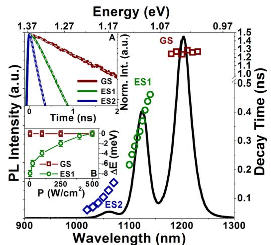
FIG. 2. Combination of power-dependent PL and TRPL experimental results measured at  $T = 10 \text{ K}$ . The peak position versus the power density for GS and ES1 is depicted in the inset B. The decay times extracted for selected wavelengths are represented by colored opened symbols. The decay profiles corresponding to each separate emission and their single exponential fits (grey dashed lines) are depicted in the inset A.
