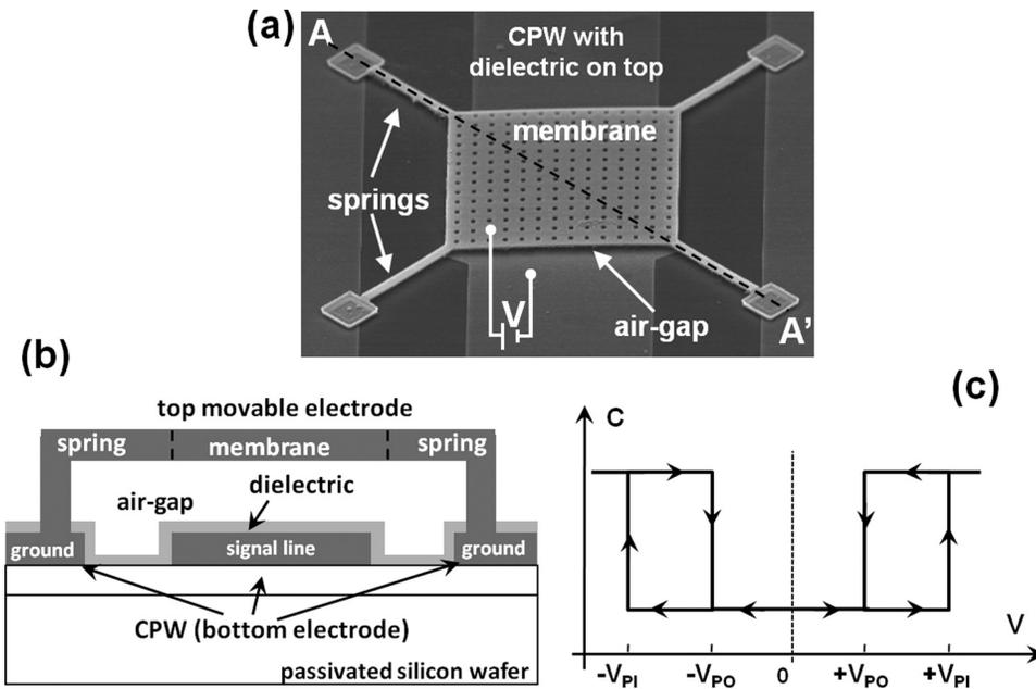
FIG. 1. (a) SEM image of a typical capacitive switch used in this work, the membrane area is  $100 \times 100 \mu\text{m}^2$ , (b) cross section along AA' cut-line, and (c) an ideal C-V characteristic of the switch.
