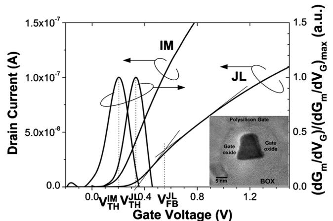
FIG. 1.  $I_D(V_G)$  characteristics of JL and IM MOSFETs and their second derivatives.  $V_D = 50$  mV. Inset: high-resolution transmission electron microscope photograph of the cross section of a transistor.
