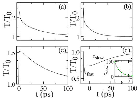
FIG. 2. (Color online) Typical pump probe dynamics for various pump/probe combinations at 1 V: (a) GS pump/GS probe; (b) ES pump/ES probe; (c) ES pump/GS probe; (d) GS pump/ES probe. (Inset) Exponential behavior of slow timescale in GS pump/ES probe case.
