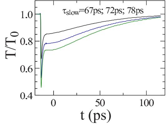
FIG. 3. (Color online) GS pump/ES probe traces at  $-2$  V for pump powers of  $100 \mu\text{W}$  (black, upper),  $190 \mu\text{W}$  (blue, middle), and  $260 \mu\text{W}$  (green, lower). The slow timescale shows a very weak dependence on pump power and can be neglected.
