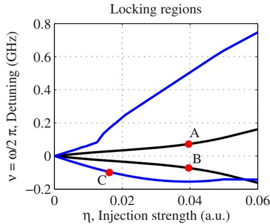
FIG. 5. (Color online) Theoretical locking regions for  $\alpha_g=0, \alpha_q=0$  (black line) and for  $\alpha_g=2, \alpha_q=0.4$  (blue line).  $g_0=0.1, q_0=3.0, \kappa=0.3, s=30.0, \gamma=30.0, \gamma_g=0.01, \gamma_q=3.0, T=10$ .
