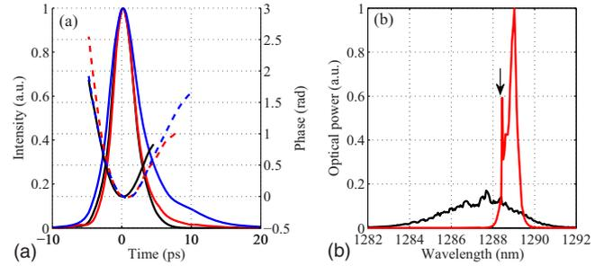
FIG. 3. (Color online) (a): Retrieved FRMZG pulses (solid lines) and phases (dotted lines) for 100 mA (narrowest), 120 mA (middle) and 130 mA (widest), absorber bias  $-6$  V. (b) Optical spectra without injection (wide) and with injection (narrow).
