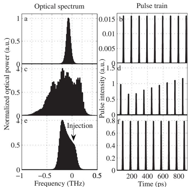
FIG. 1. Calculated pulses (b) and FTs (a) for free-running laser ( $g_0 = 0.11$ ). Calculated pulses (d) and FTs (c) for free-running laser ( $g_0 = 0.5$ ). Calculated pulses (f) and FTs (e) for injection locked laser ( $g_0 = 0.5$ ).
