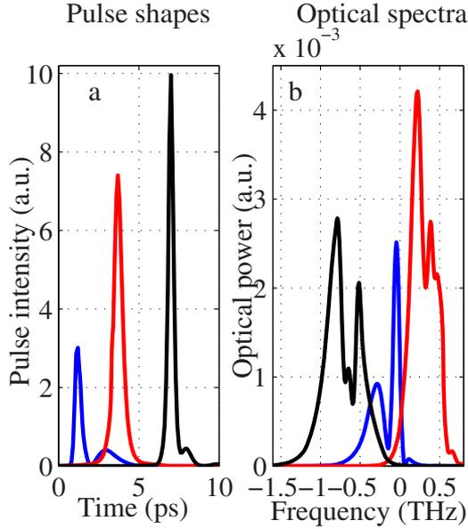
FIG. 2. (Color online) Calculated pulses (a) and FTs (b) for free-running laser ( $g_0=0.5$ ).
