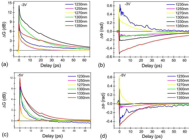
FIG. 2. (Color online) Absorption and phase recovery dynamics taken at reverse voltages of  $-3$  V and  $-5$  V. The laser's repetition rate was 80 MHz.
