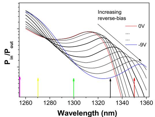
FIG. 1. (Color online) Absorption spectra of the QD waveguide absorber as a function of reverse bias voltage. Wavelengths (and voltages) at which pump probe measurements were carried out are indicated by arrows (and bold lines). In each case, the device was pumped and probed at the same wavelength.
