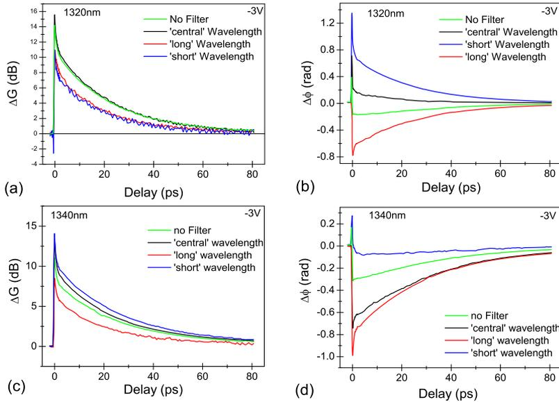
FIG. 3. (Color online) The effect of spectral filtering of the signal just before the final detector for two different central wavelengths at a reverse voltage of  $-3$  V. Different wavelength groups are selected by rotating the bandpass filter.
