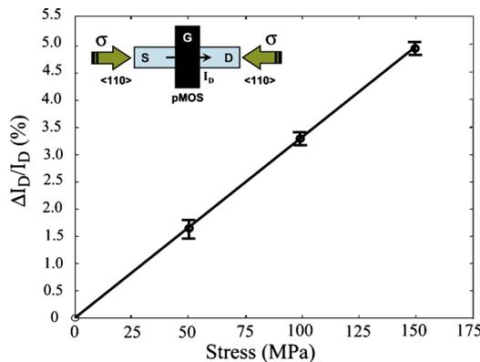
FIG. 2. (Color online) The variation in drain current,  $\Delta I_D/I_D$ , as a function of applied compression stress in a p-type junctionless MuGFET with a fin width of 30 nm.
