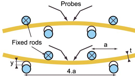
FIG. 1. (Color online) Four-point bending measurement setup and relationship between the induced stress ( $\sigma$ ) and vertical displacement ( $y$ ) of the bottom movable rods. For all measurements, the spacing “ $a$ ” was equal to 20 mm.
