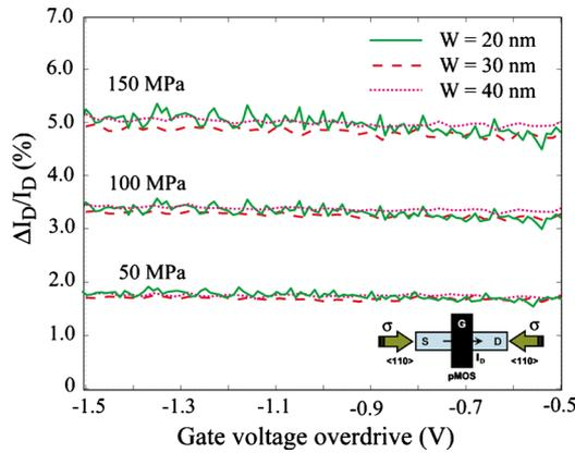
FIG. 4. (Color online) The variation in drain current,  $\Delta I_D/I_D$ , as a function of gate voltage overdrive,  $V_{GS}-V_{TH}$ , in a p-type junctionless MuGFET characterized by fin width of 20, 30, or 40 nm for various applied compressive stresses.
