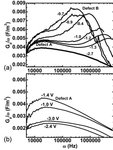
FIG. 2.  $G_p/\omega$  vs  $\omega$  ( $\omega=2\pi \times$  frequency) at  $75$  °C for selected and representative gate voltage bias points (indicated), for (a) unpassivated and (b) three-stage *ex situ* passivated Pd/10.3 nm ALD  $\text{HfO}_2/n\text{-In}_{0.53}\text{Ga}_{0.47}\text{As}/\text{InP}$ . IL thickness for the passivated  $\text{In}_{0.53}\text{Ga}_{0.47}\text{As}$  device is 1.3 nm.
