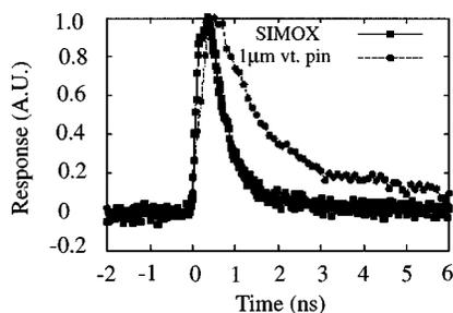
FIG. 4. Pulse response of SIMOX resonant cavity photodiode. For comparison, we also include the pulse response of a vertical  $p$ - $i$ - $n$  photodiode without the buried oxide. The vertical  $p$ - $i$ - $n$  photodiode has a much longer fall time due to a slow carrier diffusion tail due to photogeneration outside the depleted area.
