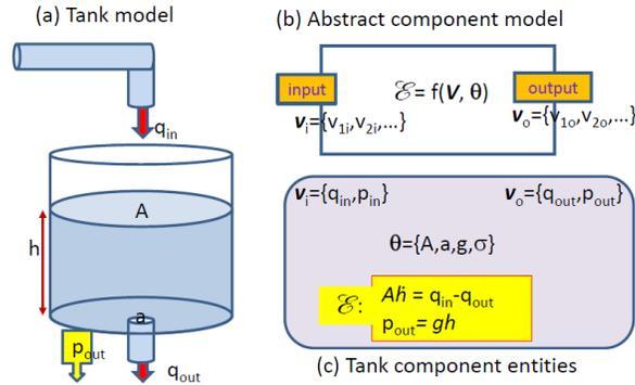
Fig. 2. Model for tank component
