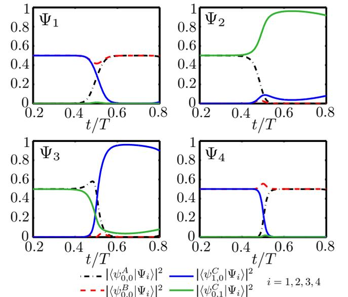
FIG. 3. (Color online) Temporal evolution of the population of each asymptotic level of the traps ( $\psi_{0,0}^A$ ,  $\psi_{0,0}^B$ ,  $\psi_{1,0}^C$ , and  $\psi_{0,1}^C$ ) for the four eigenstates of the system ( $\Psi_1$ ,  $\Psi_2$ ,  $\Psi_3$ , and  $\Psi_4$ ). The parameter values are the same as in Fig. 2.
