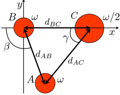
FIG. 1. (Color online) Schematic representation of the system of three harmonic traps with broken spatial symmetry. Traps A and B have a trapping frequency  $\omega$  and trap C has a trapping frequency  $\omega/2$ .
