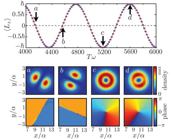
FIG. 5. (Color online) Generated angular momentum as a function of the total time of the process  $T$  (upper plot) and final states in the C trap and their phases for four different final total times *a*, *b*, *c*, and *d* (lower plots). The parameter values are the same as in Fig. 2.
