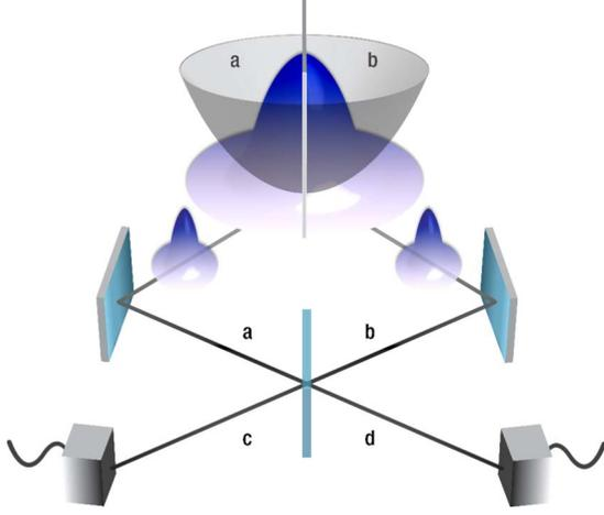
FIG. 1. (Color online) Schematic showing a trapped wave function split into two spatial modes  $a$  and  $b$ . The modes are combined at a 50:50 beam splitter and the particles in the output modes  $c$  and  $d$  are counted.
