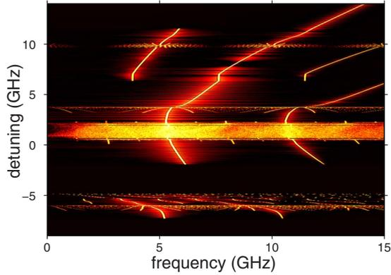
FIG. 5. (Color online) Power spectral density of the total field intensity  $|E_1|^2 + |E_2|^2$  obtained from numerical integration of Eqs. (1)–(3) as a function of the detuning. The injected field strength is  $K=0.008$ .
