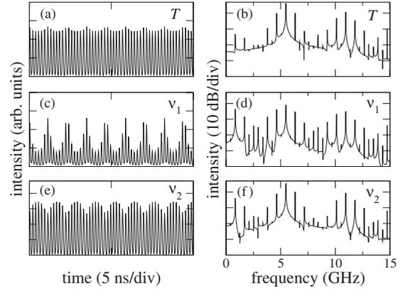
FIG. 8. Numerically computed antiphase dynamics, region (ii). The frequency detuning is 3.4 GHz. The injected field strength is  $K=0.008$ . Left panels: Intensity time traces. Right panels: Power spectral densities. [(a) and (b)] total intensity. [(c) and (d)] uninjected mode. [(e) and (f)] injected mode.
