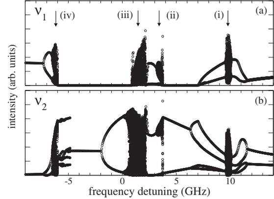
FIG. 6. Local extrema of the field intensities (a)  $|E_1|^2$  and (b)  $|E_2|^2$  obtained from numerical integration of Eqs. (1)–(3) as a function of the detuning. The injected field strength is  $K=0.008$ . Upper panel: uninjected field. Lower panel: injected field.
