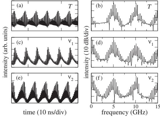
FIG. 7. Numerically computed antiphase dynamics, region (i). The frequency detuning is 10.0 GHz. The injected field strength is  $K=0.008$ . Left panels: Intensity time traces. Right panels: Power spectral densities. [(a) and (b)] total intensity. [(c) and (d)] uninjected mode. [(e) and (f)] injected mode.
