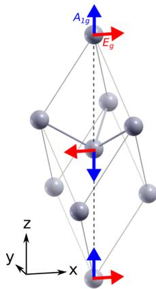
FIG. 1 (color online). The bismuth rhombohedral unit cell. The blue (vertical) and red (horizontal) arrows indicate atomic motion in the  $z$  and  $x$  Cartesian directions, corresponding to the  $A_{1g}$  and  $E_g$  phonon modes, respectively. The body diagonal (dashed line) corresponds to the  $c$  axis in the text.
