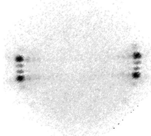
FIG. 2. Near field (top) and far field (bottom) of a single frequency standing wave of the laser intensity. The laser aperture is  $15 \times 15 \mu\text{m}^2$ . The spatial wavelength of the intensity of this pattern is approximately  $0.75 \mu\text{m}$  and the corresponding divergence in air is  $65^\circ$  full angle.
