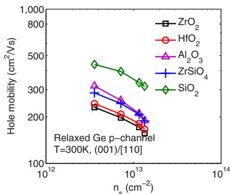
FIG. 12. (Color online) Hole mobility in relaxed Ge p-channels with a variety of gate insulators. Not surprisingly, our results show that high- $\kappa$  dielectrics affect negatively the hole mobility, compared with channels with an SiO<sub>2</sub> insulator, due to the effect of remote phonons. In addition, ZrO<sub>2</sub> and HfO<sub>2</sub> degrade hole mobility more than Al<sub>2</sub>O<sub>3</sub> and ZrSiO<sub>4</sub>.
