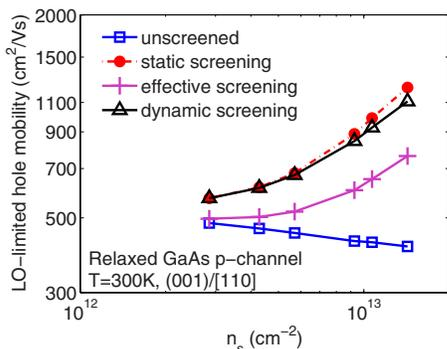
FIG. 3. (Color online) Effect of the various screening models described in the text (effective, static, and dynamic) on the LO-limited hole mobility in a relaxed GaAs p-channel with SiO<sub>2</sub> insulator. The use of the effective-screening model underestimates the hole mobility while static screening shows a modest overestimation of the LO-limited mobility.
