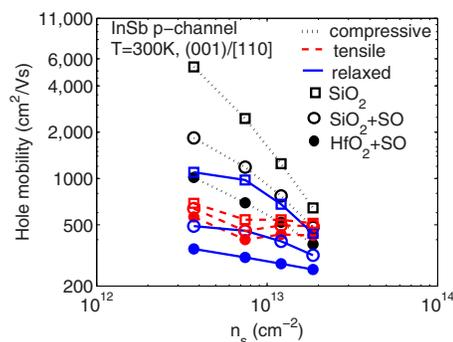
FIG. 5. (Color online) Strain-dependent hole mobility in relaxed (solid line), 2% biaxially compressed (dotted line), and 2% biaxially tensed (dashed line) InSb p-channel with SiO<sub>2</sub> (line) and HfO<sub>2</sub> (symbol) insulators. Stress is applied on the (001) surface.
