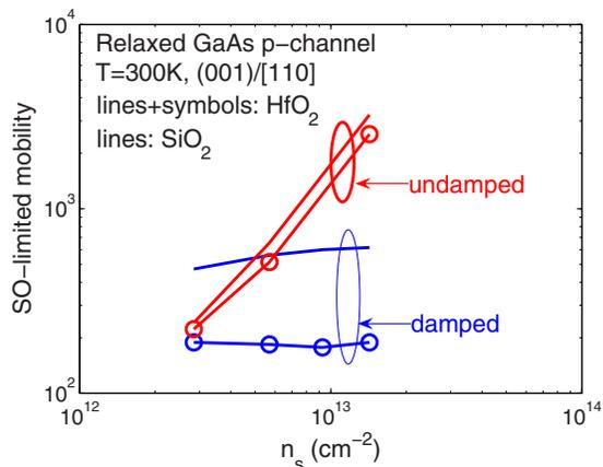
FIG. 2. (Color online) Effect of Landau damping on SO-limited hole mobility in a relaxed GaAs p-channel of a MOS system with an SiO<sub>2</sub> or an HfO<sub>2</sub> gate insulator.
