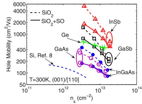
FIG. 10. (Color online) Calculated hole mobility in GaAs, GaSb, InSb,  $\text{In}_{0.7}\text{Ga}_{0.3}\text{As}$  p-channels under biaxial compressive strain and Ge channels under biaxial tensile strain with  $\text{SiO}_2$  gate insulator including (solid lines) and excluding (dashed lines) the SO phonon scattering. The Si universal curve is from Ref. 8. Biaxial stress is applied on the (001) surface.
