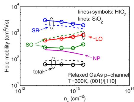
FIG. 4. (Color online) Hole mobility components in a relaxed GaAs p-channel with SiO<sub>2</sub> and HfO<sub>2</sub> insulators.
