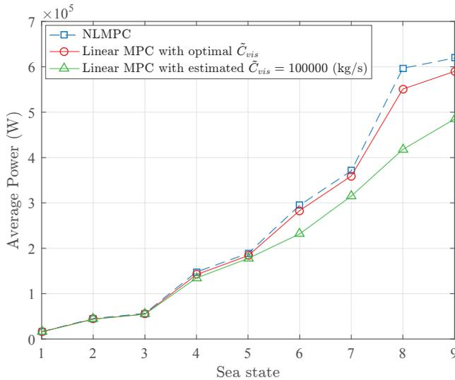
Fig. 6. A comparison of the average electrical powers found without constraints using i) NLMPC, ii) Linear MPC, where the optimally tuned  $\tilde{C}_{vis}$  estimations are used and iii) Linear MPC, with a sea state invariant  $\tilde{C}_{vis} = 100000$  (kg/s) which is constant for all sea states.
