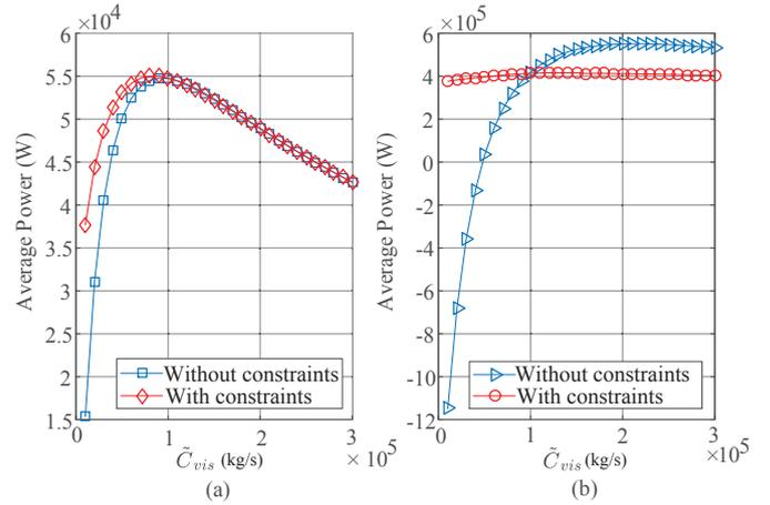
Fig. 4. Linear MPC performance with and without constraints. Average electrical power absorbed from (a) sea state 3 ( $T_s = 13.326$  s  $H_s = 1.5$  m), (b) sea state 8 ( $T_s = 13.326$  s  $H_s = 6$  m) using a Bretschneider spectrum
