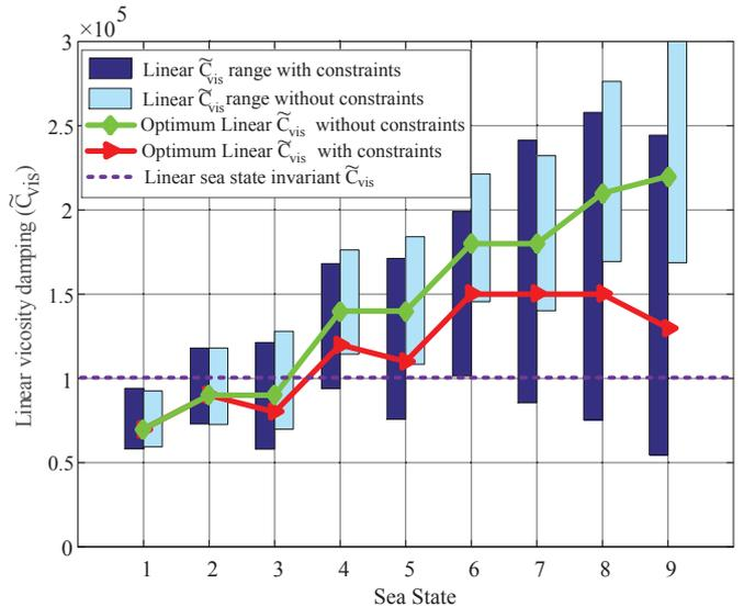
Fig. 5. The linear  $\tilde{C}_{vis}$  range of the maximum available by optimal choice of  $\tilde{C}_{vis}$  that produces an average power between 98% and 100%,  $\tilde{C}_{vis98\%}$  with and without constraints is shown. Furthermore, the optimum linear  $\tilde{C}_{vis}$  is given for each sea-state.
