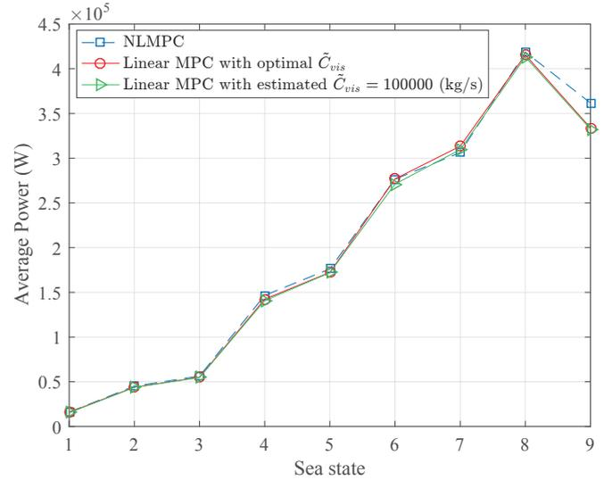
Fig. 7. A comparison of the average electrical powers found with constraints using i) NLMPC, ii) Linear MPC, where the optimally tuned  $\tilde{C}_{vis}$  estimations are used and iii) Linear MPC, with a sea state invariant  $\tilde{C}_{vis} = 100000$  which is constant for all sea states.
