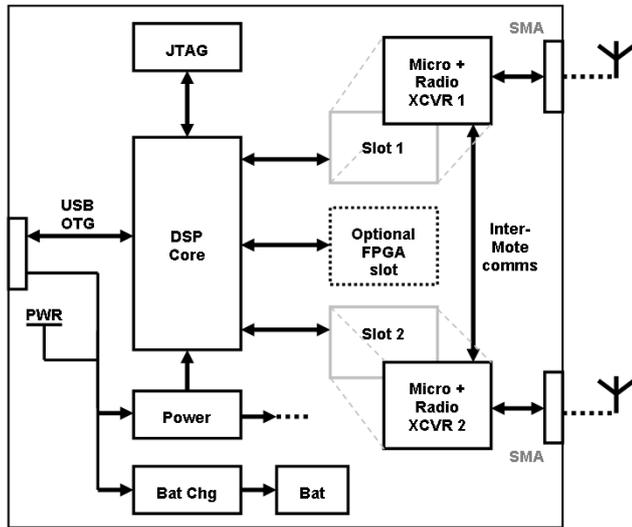
Figure 1. Block diagram of the proposed s-Mote
