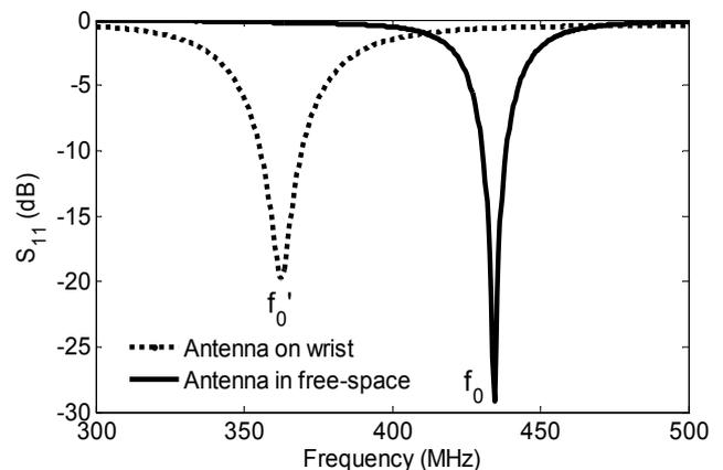
Fig. 2 Antenna detuning caused by human wrist
