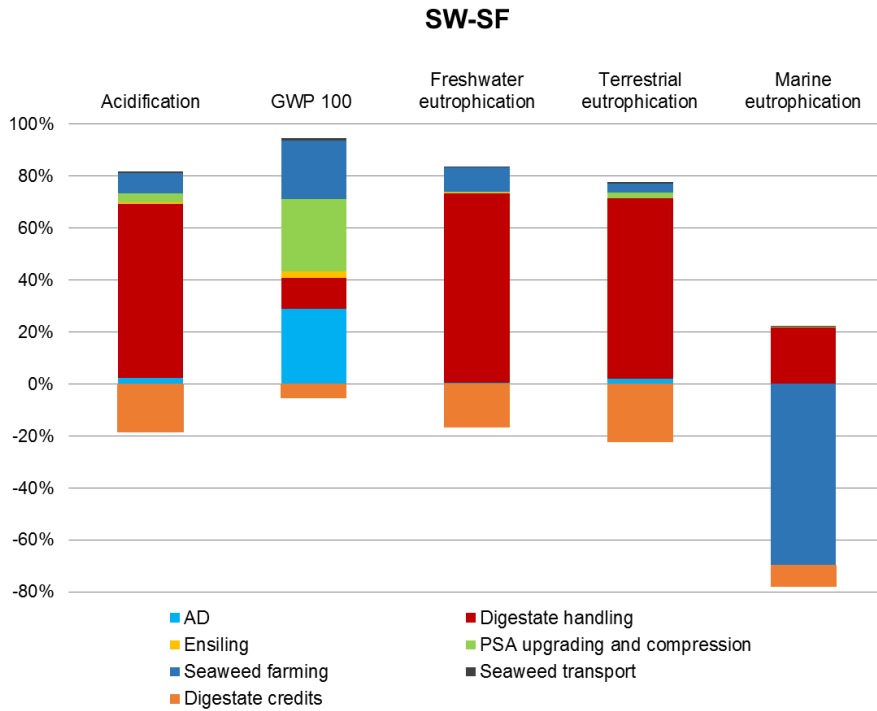
Figure 4 Cradle to gate environmental impacts of 1 MJ of biomethane from L. digitata in the baseline scenario SW-SF including both impacts and benefits from digestate (30% replacement).
