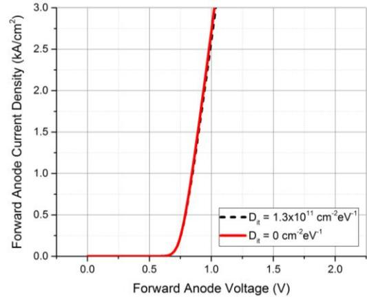
Fig. 7. Simulated forward bias characteristics of the NWSBD with a drift doping concentration of  $2 \times 10^{17} \text{ cm}^{-3}$  and effective pillar height of  $2.3 \text{ }\mu\text{m}$ . The NW diameter is 500 nm with a 500 nm inter-NW oxide gap.
