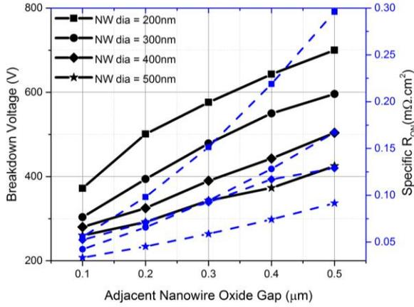
Fig. 8. Specific differential RON (dashed lines) and breakdown voltage (solid lines) for different NW diameters and oxide gap for the NWSBD. The NWSBDs have a drift doping concentration of  $2 \times 10^{17} \text{ cm}^{-3}$  and effective pillar height of  $2.3 \mu\text{m}$ .
