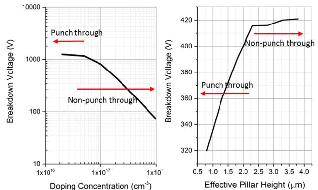
Fig 3(a) Simulated breakdown voltage dependence on the doping concentration for an effective NW height of 4.5  $\mu\text{m}$  and (b) breakdown voltage dependence on the NW height for the controlled minimum drift doping concentration of  $2 \times 10^{17}$   $\text{cm}^{-3}$ . The NW diameter is 500 nm with a 500 nm inter-NW oxide gap
