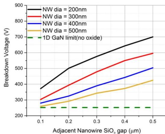
Fig. 5. Dependence of simulated breakdown voltage on NW diameter and the  $\text{SiO}_2$  gap between adjacent NWs for a drift doping concentration of  $2 \times 10^{17} \text{ cm}^{-3}$  and a height of 2.3  $\mu\text{m}$ .
