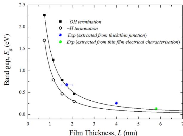
FIG. 2. Band gap versus film thickness and surface termination from *GW* calculations for Bi (111) slabs. The solid curves show a power law fit  $\alpha/L^\beta$  where  $L$  is the film thickness and  $\alpha$  and  $\beta$  are fitting parameters. The green sphere indicates experimental data ( $E_g = 125$  meV). Blue spheres are experimental estimates based on extraction from the current-voltage characteristics at different temperatures for the thick/thin junctions.
