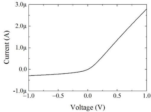
**Fig. S6** – Current voltage characteristic for the 12nm/4nm junction at T=-40 °C. The same junction is nearly Ohmic at T=+20 °C consistent with a smaller voltage barrier relative to the 12nm/1.5nm junction.
