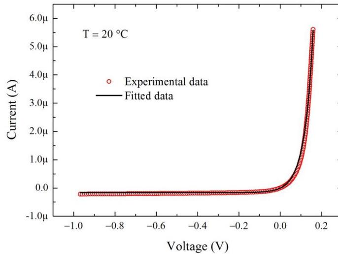
**Fig. S5** - Current-voltage (IV) characteristic of the *homomaterial* bismuth junction formed with film thicknesses 12nm/1.5nm operating near room temperature with the effects of parasitic series resistance of 150 k $\Omega$  removed.
