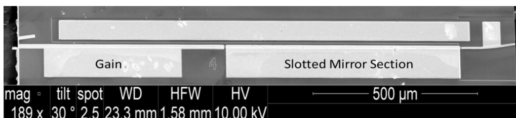
Fig 2.7: Single facet SFP laser with angled output on the right side to minimise reflections from the facet.
