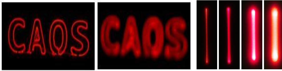
Fig. 4.4. Two sample “CAOS” lettering projections produced using two different laser pen thicknesses for text writing. Shown are also various pen thicknesses.
