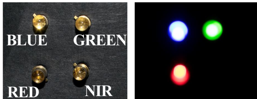
Fig. 9.2. Shown is the Visible-NIR bands target scene created using 3 visible LEDs and 1 NIR LED. Photos show LEDs off (left) and LEDs on (right). These photos are taken with a Nikon D3300 DSLR visible camera.
