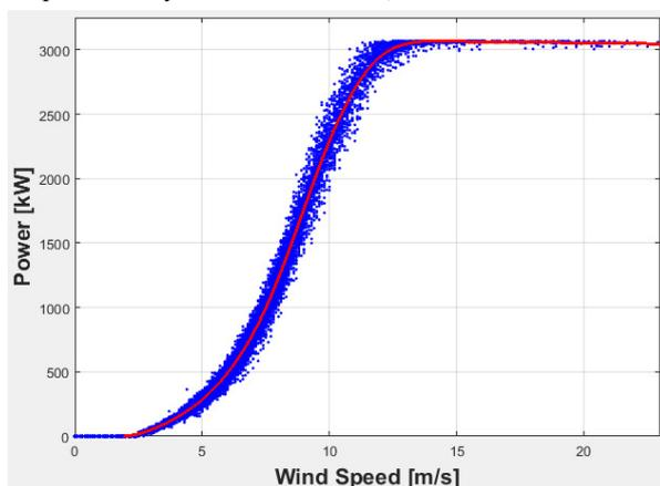
Fig. 2. Smoothing spline wind turbine power curve fitting.
