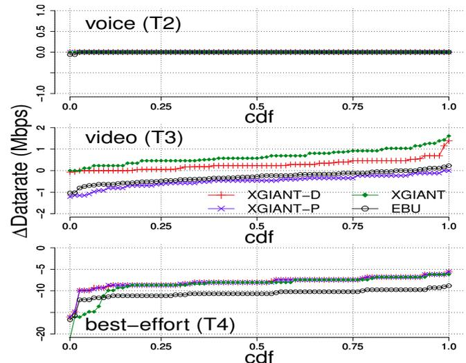
Fig. 12. Difference in mean datarate in 80-eNB scenario
