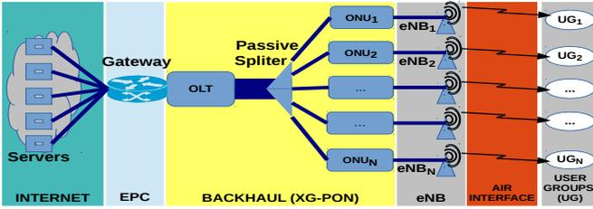
Fig. 1. Architecture of LTE network with XG-PON backhaul
