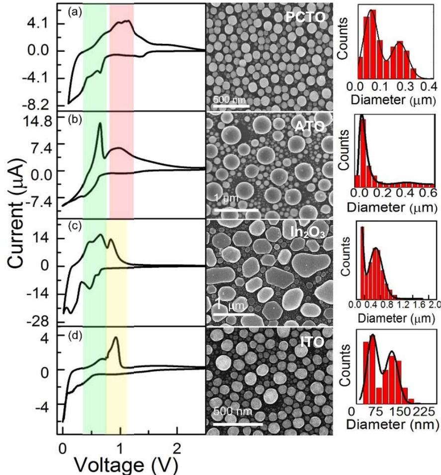
**Figure 4.** Single cycle voltammograms, SEM image of the surface of the NP layer, and corresponding size dispersion histogram for (a) PCTO NPs, (b) ATO NPs, (c) In<sub>2</sub>O<sub>3</sub> NPs, and (d) Sn-doped In<sub>2</sub>O<sub>3</sub> (ITO) NPs. De-intercalation potential windows are shaded for Li<sub>x</sub>Si (green), Li<sub>x</sub>Sn (pink) and Li<sub>x</sub>In (yellow).
