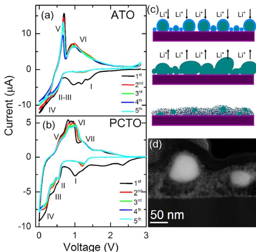
**Figure 3.** (a) Cyclic voltammograms for ATO and (b) PCTO NPs on silicon. (c) Schematic diagram describing formation of porous NP layers upon lithiation cycling. (d) Dark-field STEM image showing highly porous layer comprising pulverized NPs formed by electrochemical cycling of the PCTO NP layer. The brighter regions are Sn and SnO<sub>2</sub>.
