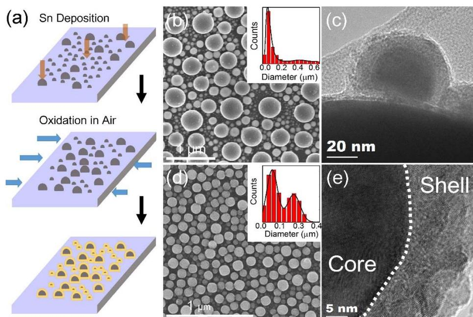
**Figure 1.** (a) Schematic diagram highlighting steps in formation of core-shell SnO<sub>2</sub> NPs. (b) SEM image showing the ATO NP dispersion. Inset shows the diameter distribution for ATO NPs. (c) TEM image of NPs grown hierarchically on the surface of ATO NP. (d) SEM image of PCTO NP layer. Inset: diameter distribution histogram for PCTO NP layer. (e) TEM image of NPs grown hierarchically on the surface of ATO NP.
