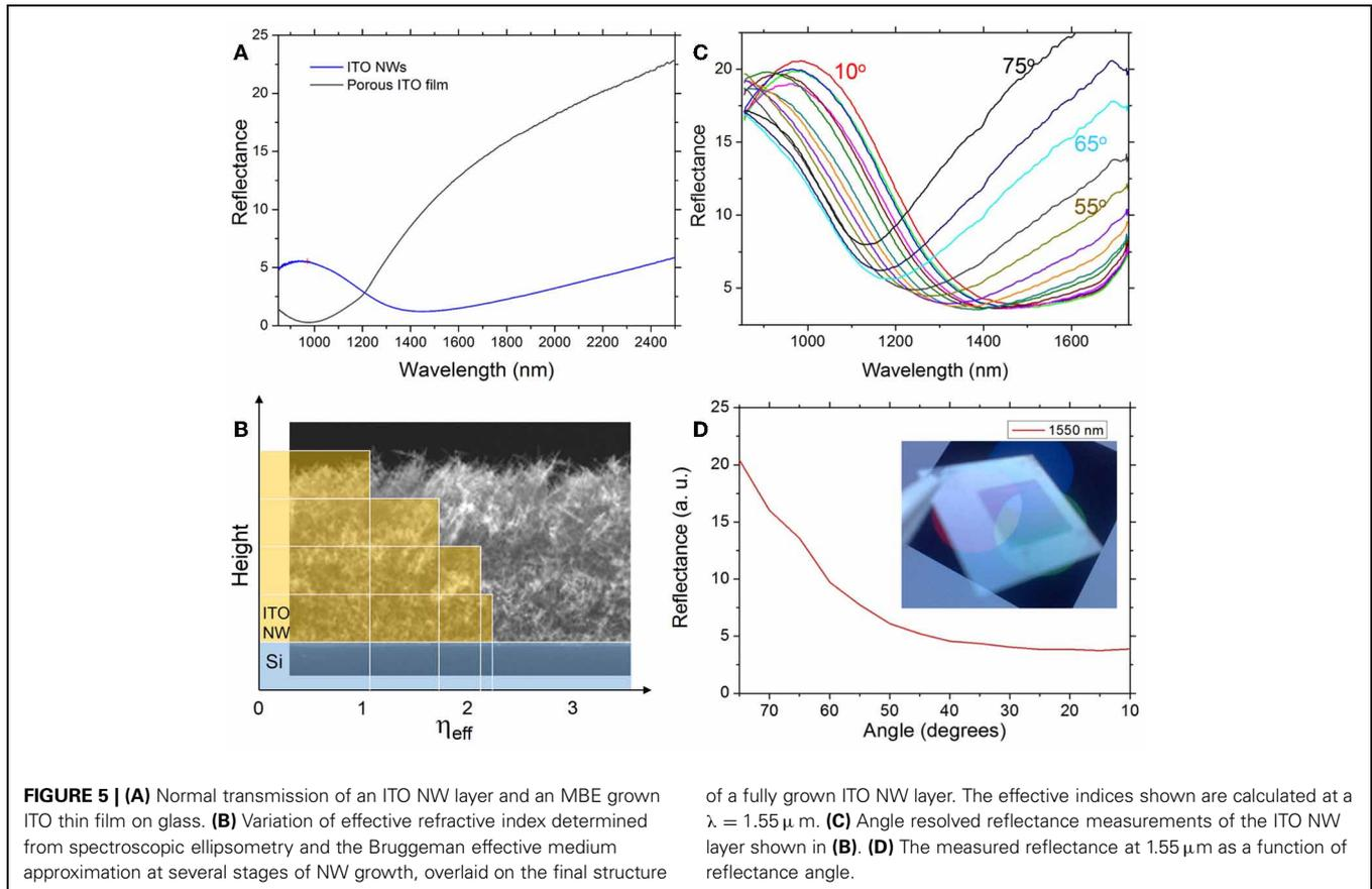
on the NW size, distribution, branching and overall optical morphology. The low refractive index NW layer is optically specular and exhibits a darker surface, confirming the absence of Fresnel reflection over a broad spectral width. This is particularly important for LED applications because of the isotropic emission from the active region and the fact that reflection phenomena can limit the light-extraction efficiency (27, 38, 39).
