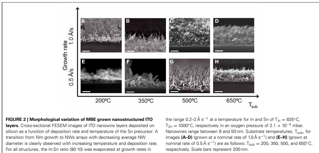
so that morphology differences are specifically a function of the deposition parameters and not variations in vapor transport and condensation for a given set of parameters. A transition from thin film to porous thick film to high aspect ratio NW layers is characteristically found at higher substrate temperatures and deposition rates for In:Sn ratios nominally of 90:10.
