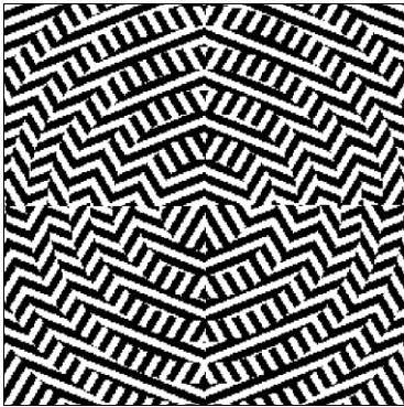
Fig. 9 Microrelief pattern of a metalens in transmission to simultaneously perform linear-to radial polarization conversion and focus light. [11]
