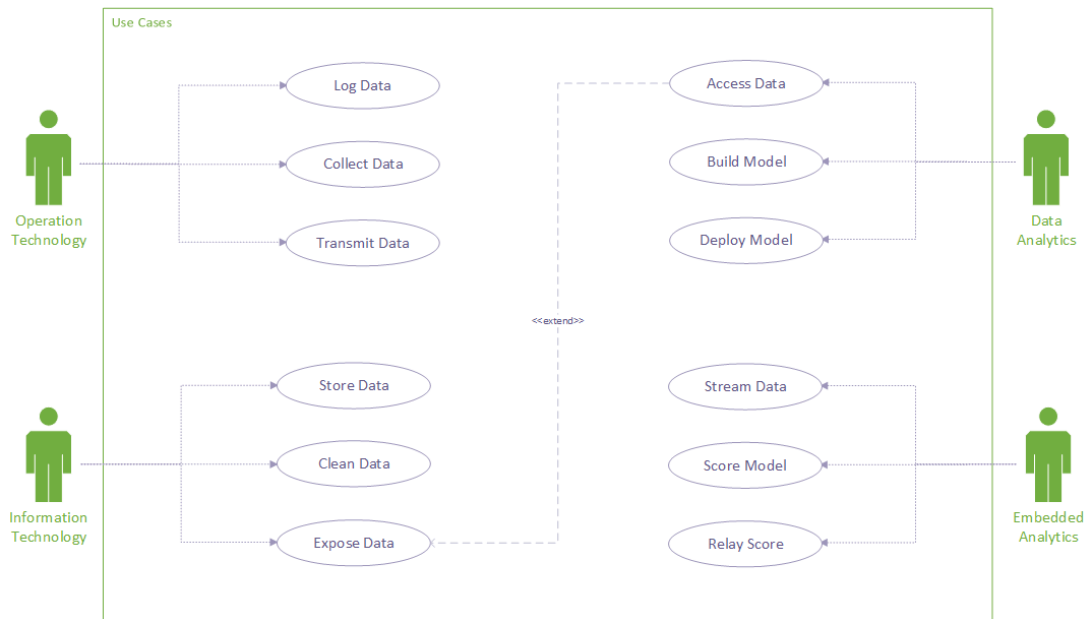
Figure 43 Primary use cases extracted from conceptual model
