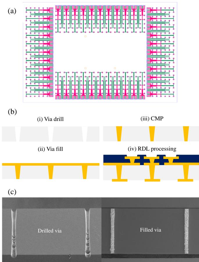
Fig. 7. (a) Design of the TGV interposer, in which the red denotes layer 1 and green layer 2 RDLs, (b) TGV interposer fabrication flow and (c) SEM images of drilled and filled TGVs.
