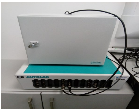
Fig. 3. Laboratory based tabletop potentiostat, the Autolab PGSTAT302N.
