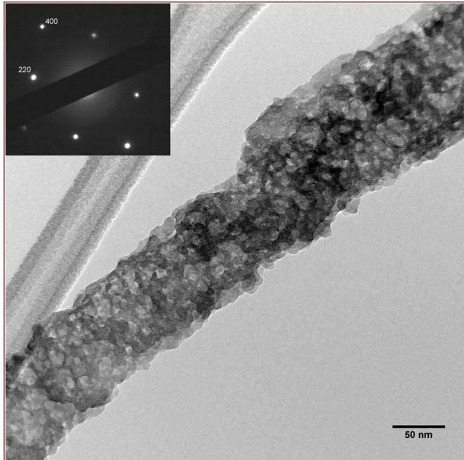
**Fig. 4** (Colour) TEM image of a rough Si nanowire prepared by the one-step MAE process along with the SAED pattern (inset) showing the  $\langle 100 \rangle$  etch direction of the wires formed.
