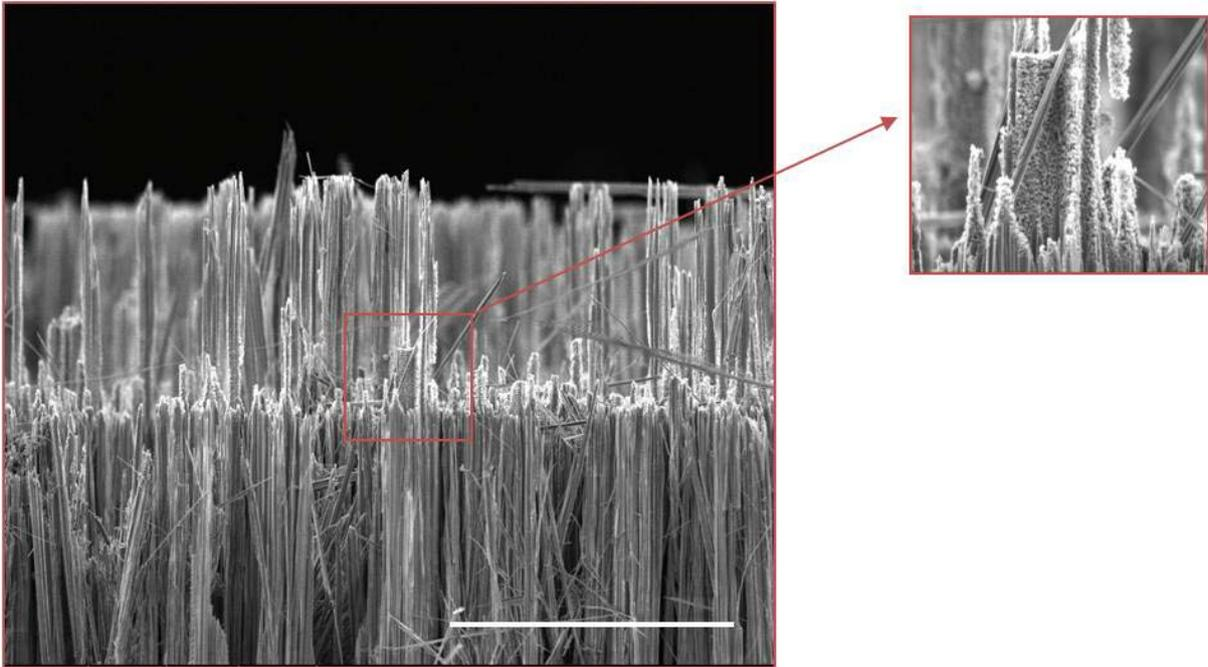
**Fig. 1**(Colour) SEM image of a Si substrate immersed for 2 h in an etching solution containing  $[AgNO_3] = 0.08$  M and 12 % HF at a temperature of 50 °C. The Si nanowires are porous to the depth of the step. Scale bar is 30  $\mu$ m.
