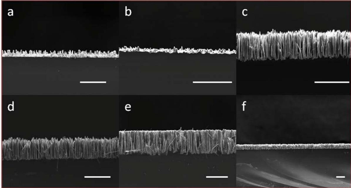
**Fig. 3** (Colour) SEM images of Si substrates immersed for (a) 10 min (b) 30 min (c) 60 min (d), (f) 90 min and (e) 120 min in an etching solution containing  $[\text{AgNO}_3] = 0.04 \text{ M}$ , 5 % HF solution at a temperature of  $50 \text{ }^\circ\text{C}$ . All scale bars are  $30 \text{ }\mu\text{m}$ .
