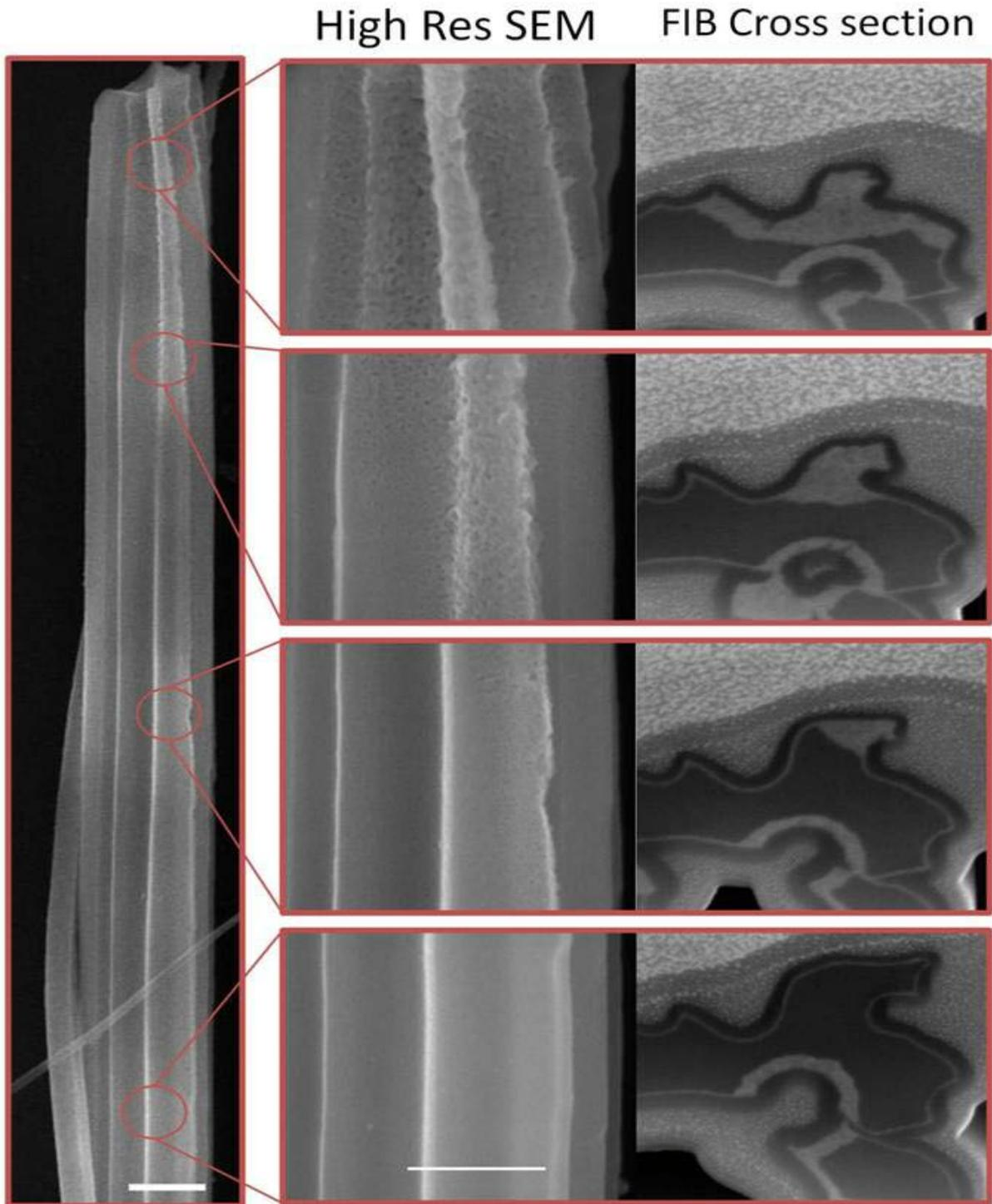
**Fig. 5** (Colour) Left: high resolution SEM image of a MAE Si nanowire produced by the one-step process. Scale bar is 200 nm. Right: high resolution SEM plan and cross sectional view of the same Si nanowire from porous region (top) to non-porous region (bottom). (Scale bars = 200 nm)
