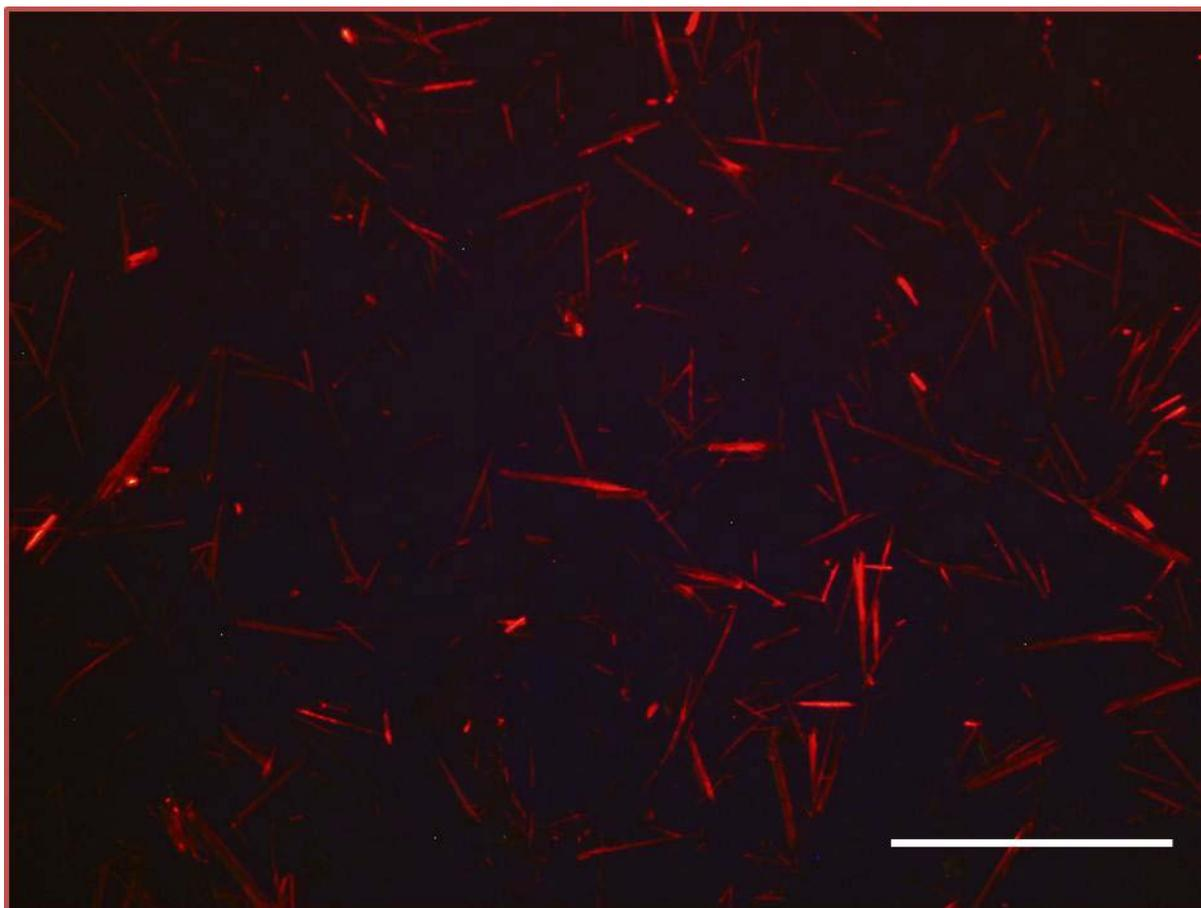
**Fig. 6** (Colour) MAE Si nanowires functionalised with dye-conjugated streptavidin. The fluorescing seems to be stronger at one end of the nanowires. Scale bar is 200 nm.
