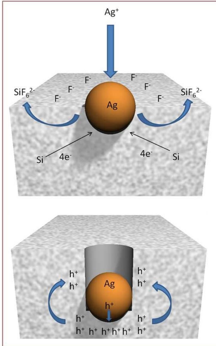
**Fig. 2** (Colour) Schematic illustrating how Si nanowire porosity results from hole migration during the one-step metal assisted etching process.
