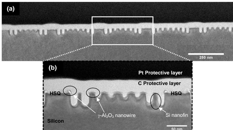
**Figure 3.** (a) Cross-section TEM image of large area of Si nanofins following pattern transfer of alumina nanowire hardmask in  $\sim 265$  nm pitch HSQ trenches. (b) High resolution TEM image of Si nanofins between HSQ gratings where the reduced Si nanofin feature size and increased etch depth at the HSQ sidewalls is evident.
