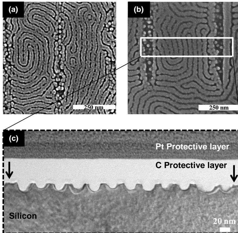
**Figure 4.** Top-down SEM images of Si nanofins in HSQ trenches of (a) ~ 285 nm and (b) ~ 350 nm respectively. (c) Cross-section TEM of Si nanofins fabricated from alumina nanowires acting as a hardmask in HSQ trenches. The pitch of the HSQ trenches was 350 nm. Arrows in (c) indicate where HSQ gratings were prior to etching. With a larger HSQ pitch and slightly increased commensurability compared to the ideal ( $32n$ ), reduced features were not observed at the sidewalls.
