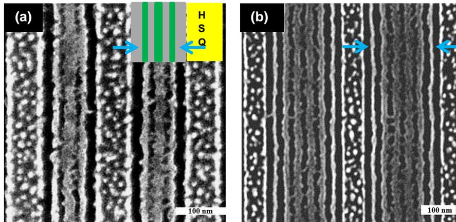
**Figure 2.** Top-down SEM image of (a) 3 Si nanofins within 128 nm HSQ gratings and (b) 6 Si nanofins within 224 nm HSQ gratings. Nanofins aligned next to the HSQ gratings show reduced feature sizes in comparison to the remaining Si nanofins. Green lines in (a) represent Si nanofins. Arrows in (a) and (b) point to the reduced feature sizes of nanofins next to HSQ gratings.
