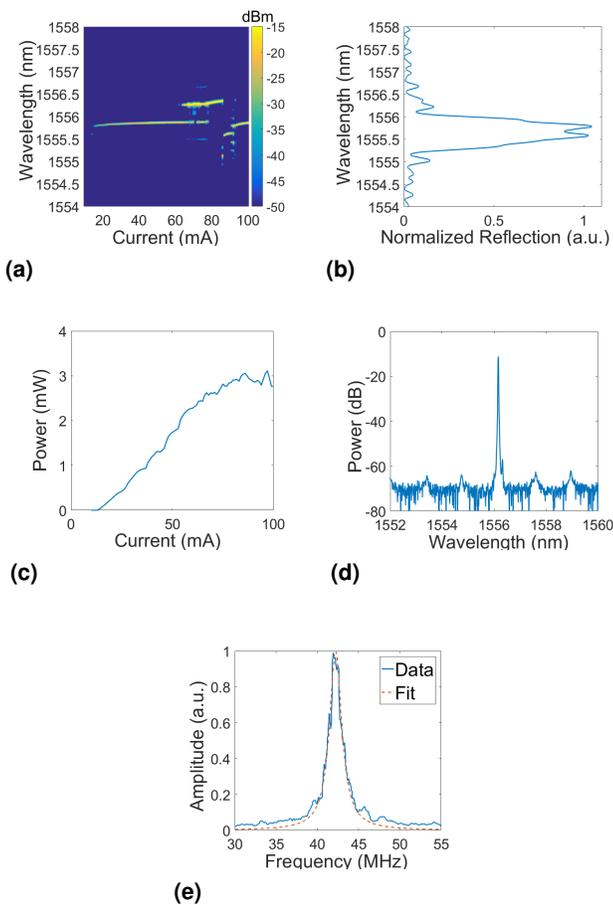
**Fig. 4.** Laser characterization. (a) False colour plot of the optical spectrum of the laser, averaged in time, with the increasing driving current. (b) Normalized reflection spectrum of the Bragg gratings, with the wavelength axis matched to that on the left, (c) L-I curve of the EC laser. (d) Time-averaged optical spectrum of the EC laser at room temperature and 50 mA of driving current. The laser line shows 49 dB of SMSR. (e) Linewidth of the hybrid EC laser and fit.
