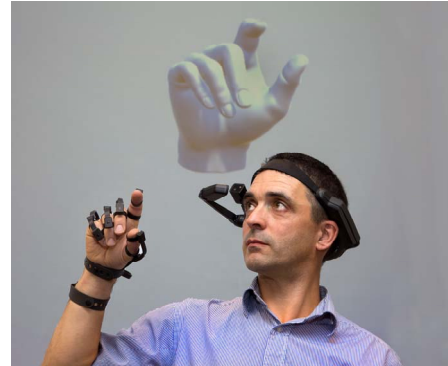
Fig. 2 System demo (data glove + Unity 3D VR platform)
