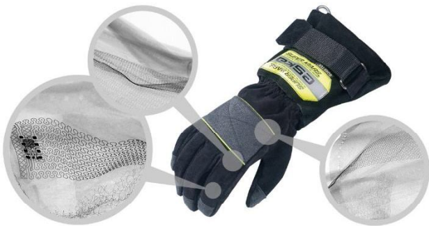
Figure 4. SAFESENS Firefighter Glove Demonstrator: X-ray images of the Textile-integrated Stretchable Electronic System
