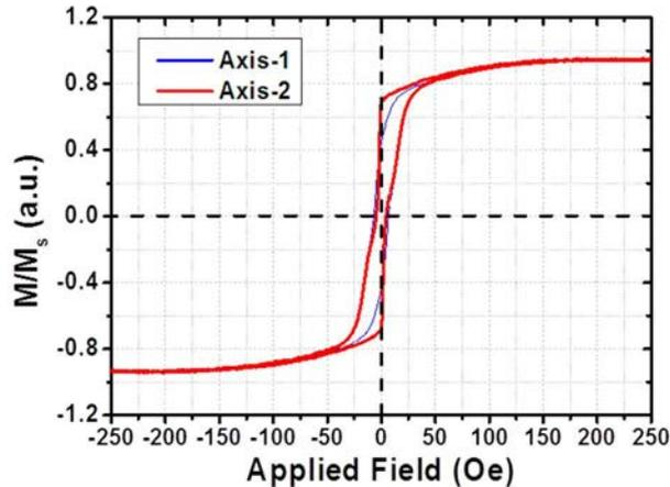
Fig. 7. Hysteresis curve of 100 nm permalloy deposit.
