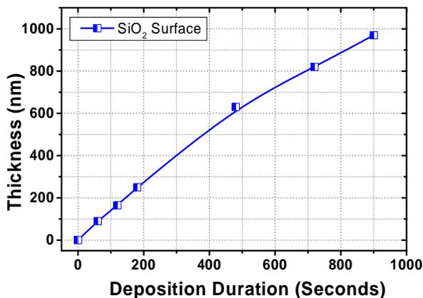
Fig. 4. Deposition rate of permalloy deposits on SiO<sub>2</sub> surface.
