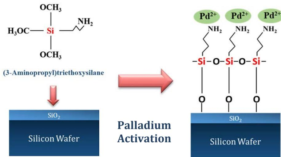
Fig. 3. Schematics of self-assembled monolayer deposition process and Pd<sup>2+</sup> deposition as catalyst layer.
