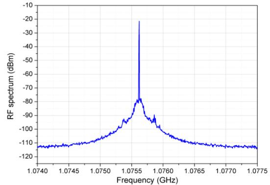
Figure 4. RF spectrum of the output pulses. The repetition rate of 1.0755 GHz is in agreement with the cavity length.
