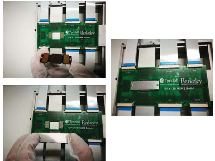
Fig. 5. Board level demonstration of the pluggable package.
