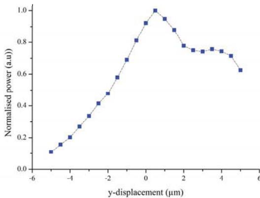
Fig. 12. Insertion loss between a pair of vertically stacked gratings in the along (y-) direction at  $z = 20 \mu\text{m}$ .
