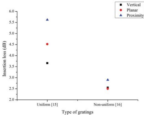
Fig. 7. 2D-FDTD simulation comparing insertion losses of fibre-to-gratings and proximity coupling. Asymmetric and symmetric mode profiles from uniform and non-uniform gratings affect insertion losses.
