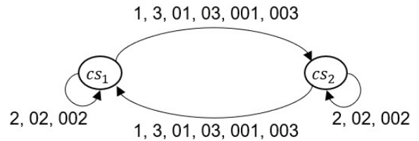
Fig. 2: A reduced finite state transition diagram based on the basic transition word set (BTWS).
