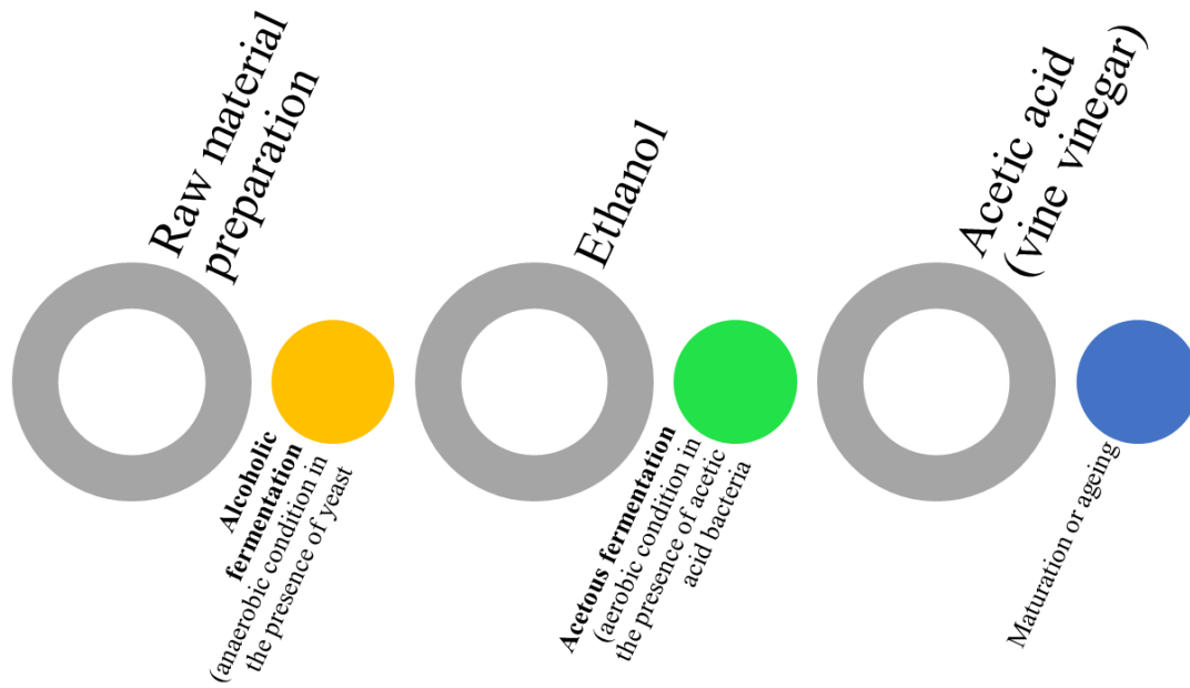
2888 Figure 3. The process of wine vinegar-making from grape juice.
