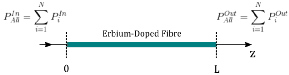
Figure D.1: Model of an erbium-doped fibre supporting N channels [227] .
