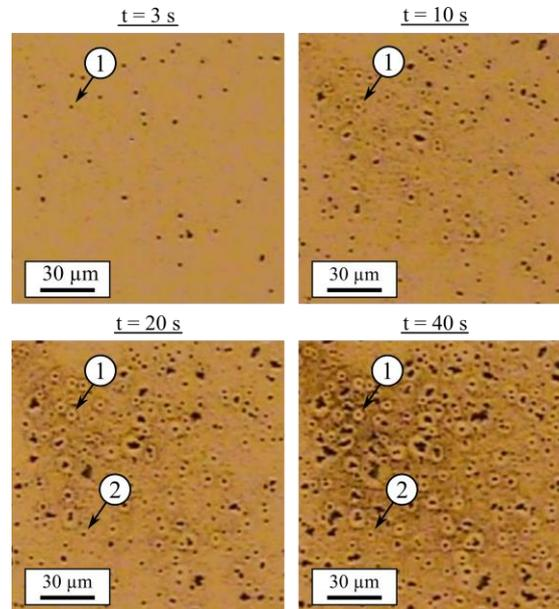
Figure 2. Optical zoom-in images of the top electrode of a Pt/HfO<sub>2</sub>/Pt device during the application of -10 V for different degradation times. The size of the images is 150μm × 150μm.
