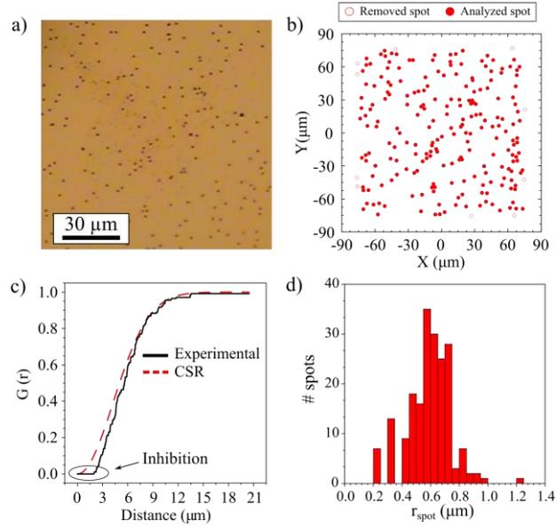
Figure 6. (a) Optical zoom-in image of a device after a CVS of 65 s. The size of the image is  $150\mu\text{m} \times 150\mu\text{m}$ . (b) Location of the spots shown in (a). The spots that are outside the observation window are not considered in the analysis. (c) Nearest-neighbour function  $G$  for the experimental data and for a CSR process. (d) Histogram for the radius of the spots.
