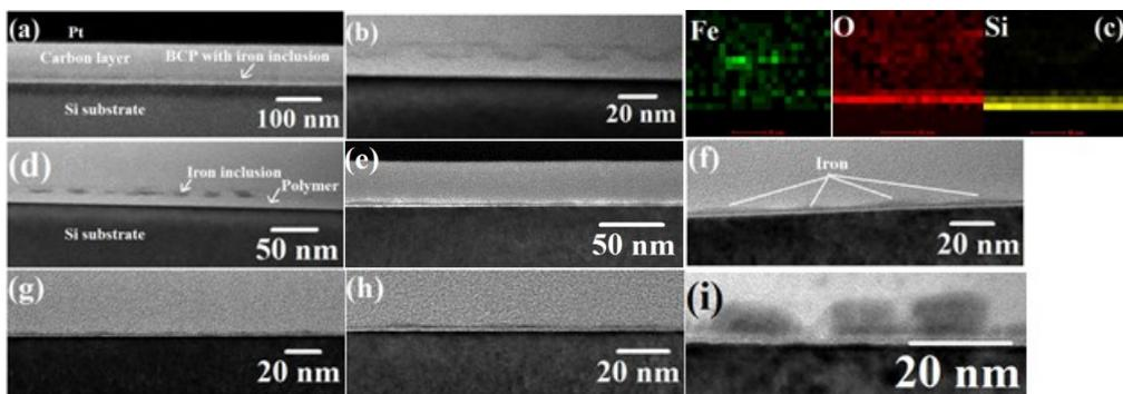
**Figure 5.** (a, b) FIB thinned TEM images and (c) EDAX mapping for Fe, O and Si after 5 min UVO exposure time. Similar data following UVO exposure times of (d) 10 min, (e, f) 30 min, (g) 1h, (h) 1h 30 min and (i) 2h 30 min.
