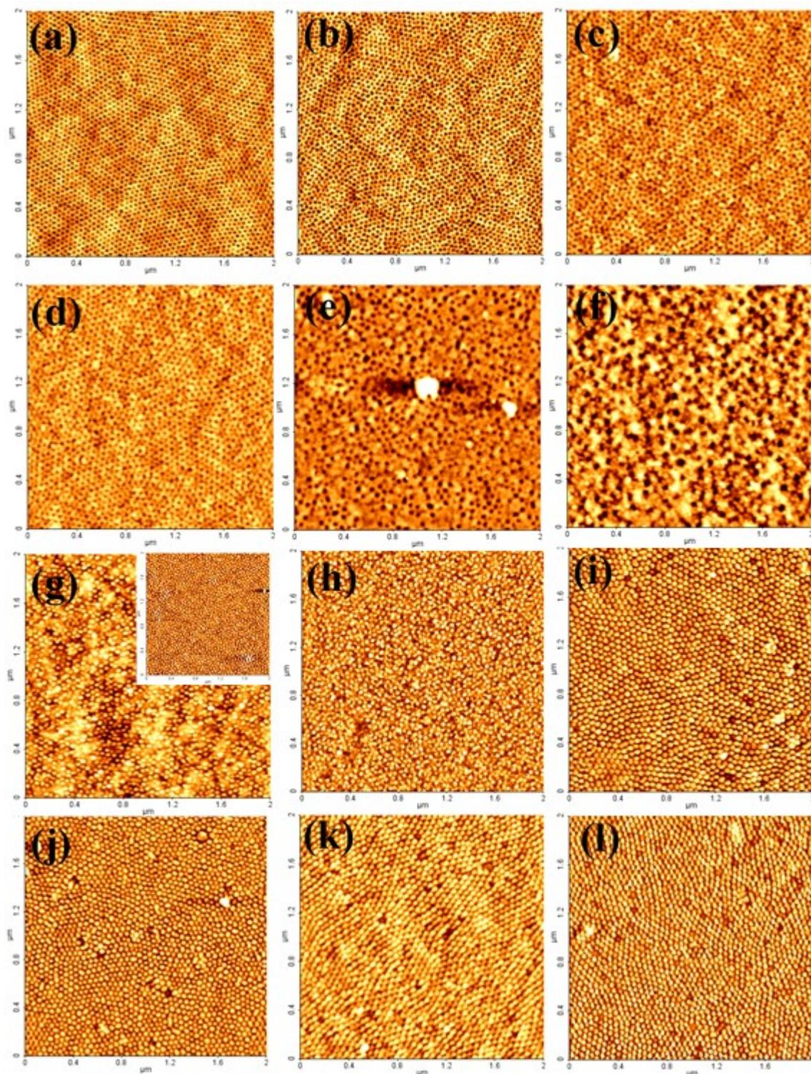
**Figure 1.** Tapping mode AFM images of the PS-b-PEO film (a) after the solvent vapour exposure, (b) after the ethanol treatment and (c) after spin coating the iron precursor. The iron oxide-BCP film for different UVO exposure time (d) 5 min, (e) 10 min, (f) 15 min, (g) 20 min, (inset of g) 25 min, (h) 30 min, (i) 45 min, (j) 1h, (k) 1h 30 min, (l) 2h.
