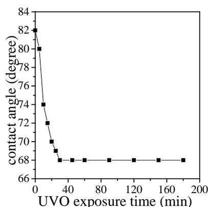
**Figure 7.** Variation of water contact angle with UVO exposure time.
