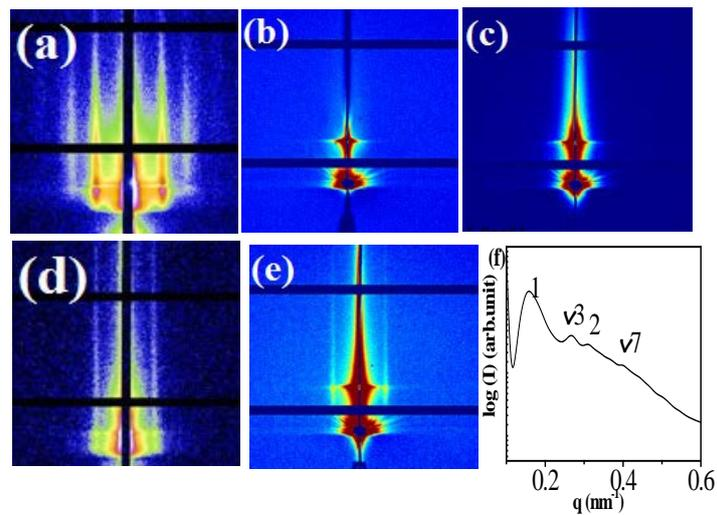
**Figure 4.** GISAXS 2D scattering spectra for UVO processing time of (a) 5 min, (b) 10 min, (c) 15 min, (d) 20 min and (e) 45 min respectively. (f)  $q_y$  line scan profile for 45 min UVO exposure time.
