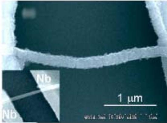
**Figure 4.** A suspended Co-doped  $\text{TiO}_2$  nanowire junction between Nb electrodes. Inset figure represents the suspended molecular template junction before fabrication of Co-doped  $\text{TiO}_2$  nanowire. Reproduced with permission from Appl. Phys. Lett. **86**, 033110 (2005). Copyright 2005, American Institute of Physics.
