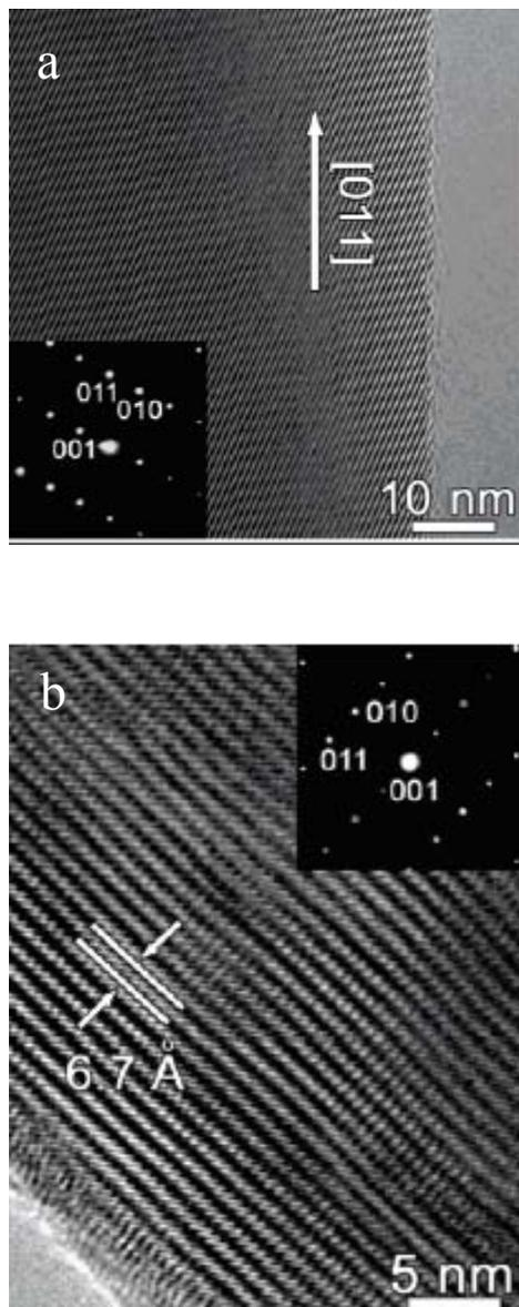
**Figure 1.** Atomic-resolved TEM image of  $\text{Cd}_{0.7}\text{Mn}_{0.3}\text{S}$  nanowires grown in the a)  $[011]$  and b)  $[010]$  growth directions. Reproduced with permission from *J. Phys. Chem B*, **110**, 6699 (2006). Copyright 2006, American Chemical Society.
