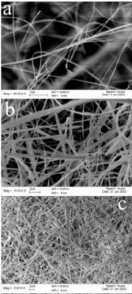
**Figure 3.** SEM images of the  $Zn_{1-x}Mn_xS$  nanowires obtained from different Zn:Mn ratios. a) Zn/Mn = 4/1 b) Zn/Mn = 8/3 c) Zn/Mn = 2/1. Reproduced with permission from Adv. Funct. Mater. **15**, 303 (2005). Copyright 2005, Wiley-VCH Verlag GmbH & Co
