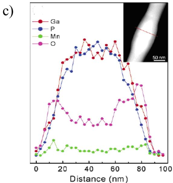
**Figure 6.** a) Detailed feature of a bumpy Mn doped GaP nanowire and its b) atomic-resolved HVEM image showing a number of defect lines along the [111] direction. c) elemental mapping cross-section showing that Mn and O concentrations at the outer layers. The corresponding STEM image is shown in the inset. Reproduced with permission from *J. Phys. Chem. B* **109**, 9311 (2005). Copyright 2005, American Chemical Society.
