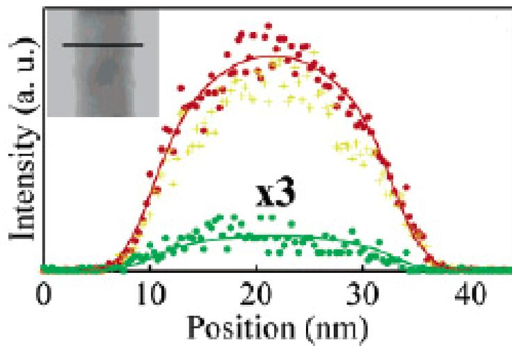
**Figure 2.** EDX line scans for the nanowire shown in the inset, with Cd, S, and Mn data plotted as red dots, yellow crosses, and green dots, respectively. The red and green solid lines through the data are fits to the experimental data for Cd and Mn, respectively. Reproduced with permission from Nano Lett. **5**, 1407 (2005). Copyright 2005, American Chemical Society.
